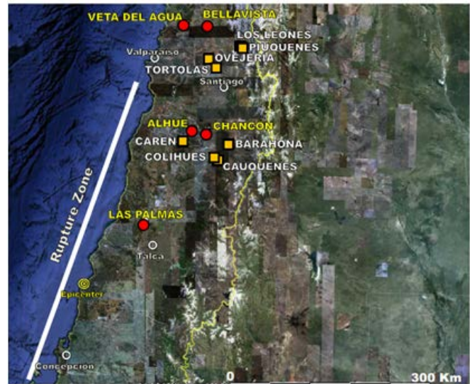
Figura 3. Zona de Ruptura sismo Maule y ubicación de Tranques de Relaves. Con círculos se indican los tranques que fallaron y con cuadrados los que no presentaron fallas (Verdugo et al., 2010). Figure 3. Fault zone and tailings dams. The tailings dams which were damaged are indicated with circles and those that were not damaged are indicated with squares (Verdugo et al., 2010).
